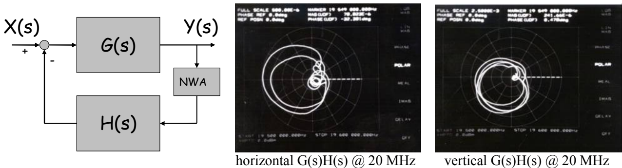
Figure 4: Results of beam transfer function measurement with feedback.
